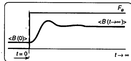
FIG. 1. Response of a phase function B to a constant field F_e applied at t=0 . The phase space average \langle B \rangle changes from its equilibrium value \langle B(0) \rangle , through transient behavior toward a constant steady-state value \langle B(t \rightarrow \infty) \rangle .
